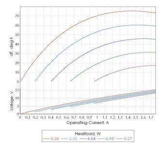
**Note**: Performance data is specified at optimal optimal conditions (TEC hot side is stabilized at ambient temperature). Any heatsink thermal resistance is not included into estimations. Use TECCad Software for estimations under different conditions.
