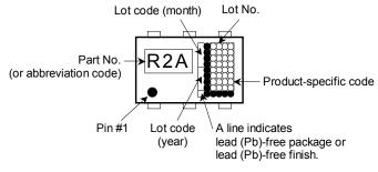
The round black marking "●" located on the lower left of the parts number marking "R2A" indicates terminal No. 1.
