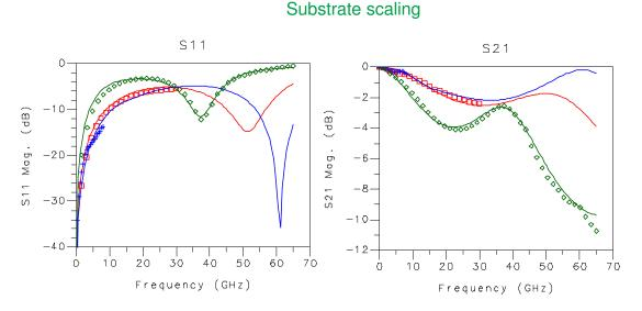
Legend: 4mil Rogers 4350B, +60mil Rogers 4003, 5mil Alumina, Lines - Model, Symbols - Measured data. Measured data stops at highest valid frequency for each substrate (4 mil - 30 GHz, 60 mil - 8 GHz, 5 mil Alumina - 65 GHz). Note: The pad dimensions used for the plots are: PADL = 15.5mil, PADW = 28.0mil, PADG = 16.0mil
