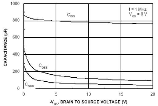
Figure 8. Capacitance Characteristic
