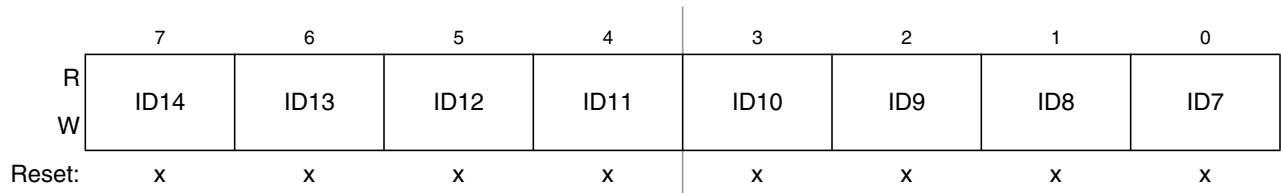
Figure 16-28. Identifier Register 2 (IDR2) — Extended Identifier Mapping
