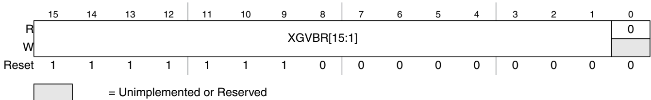
Figure 10-9. XGATE Vector Base Address Register (XGVBR)
