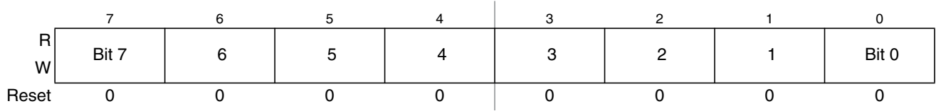
Figure 19-11. PWM Scale A Register (PWMSCLA)
