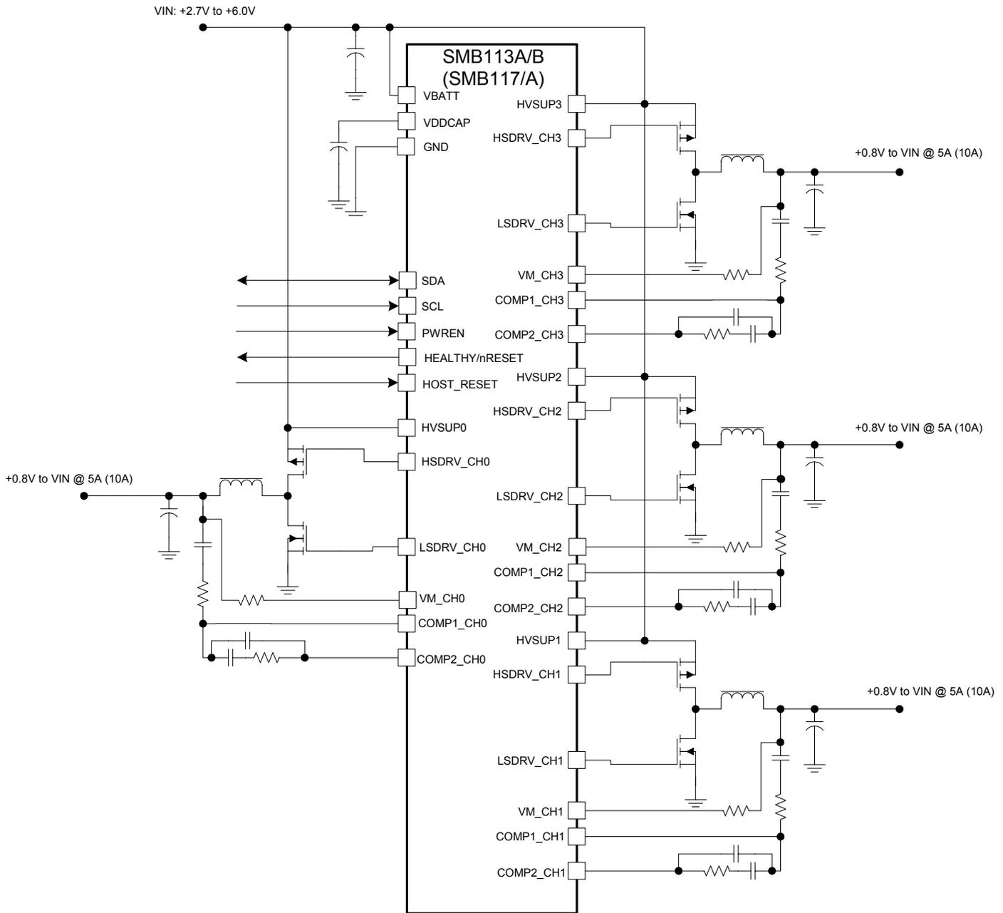
Figure 2 – Typical application schematic
