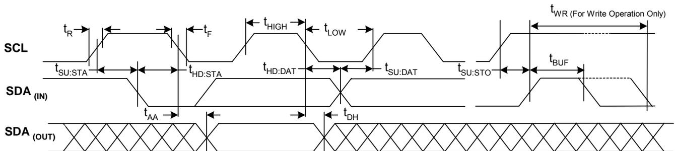
Figure 4 – I<sup>2</sup>C timing diagram
