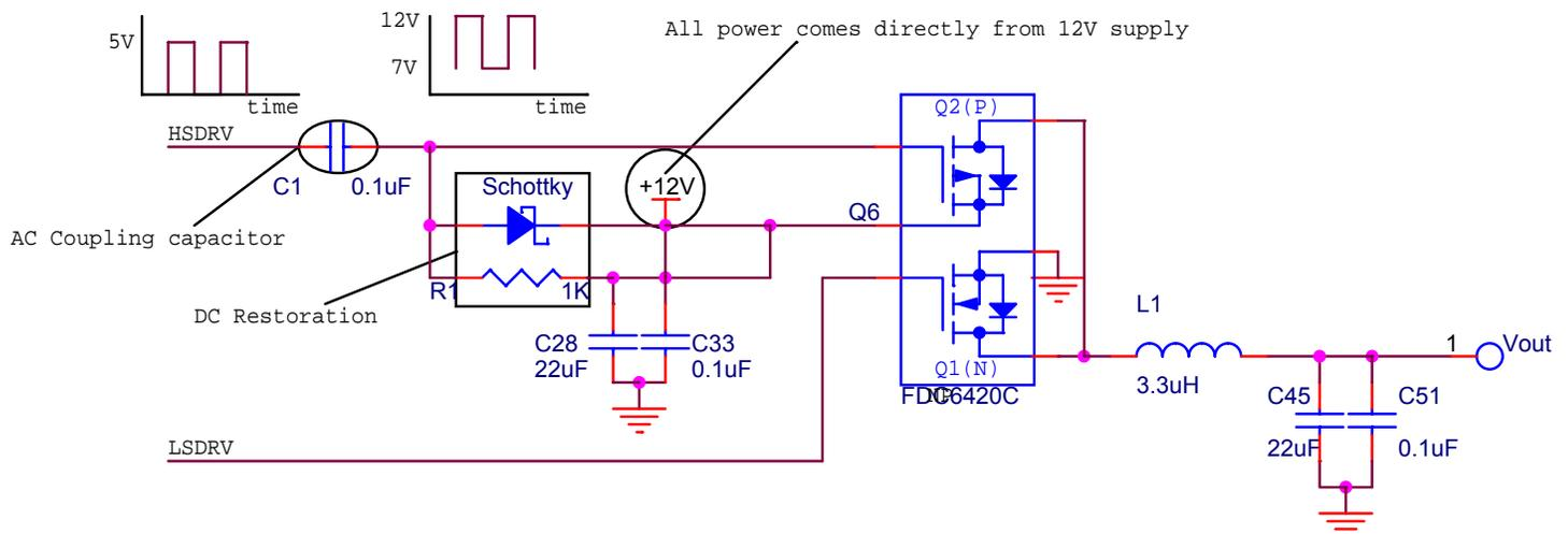
Figure 7 – High-voltage operation
