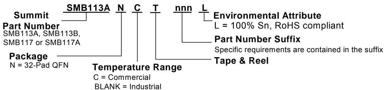
The default device ordering number is SMB113ANC-650L. It is tested over the commercial temperature range. The ordering number is derived from the customer supplied hex file. New device suffix numbers are assigned to non-default requirements.
