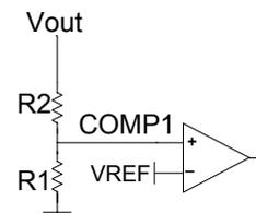
$$\text{Soft-Start Slew Rate} = \text{SRref} * (1 + \text{R2/R1})$$
