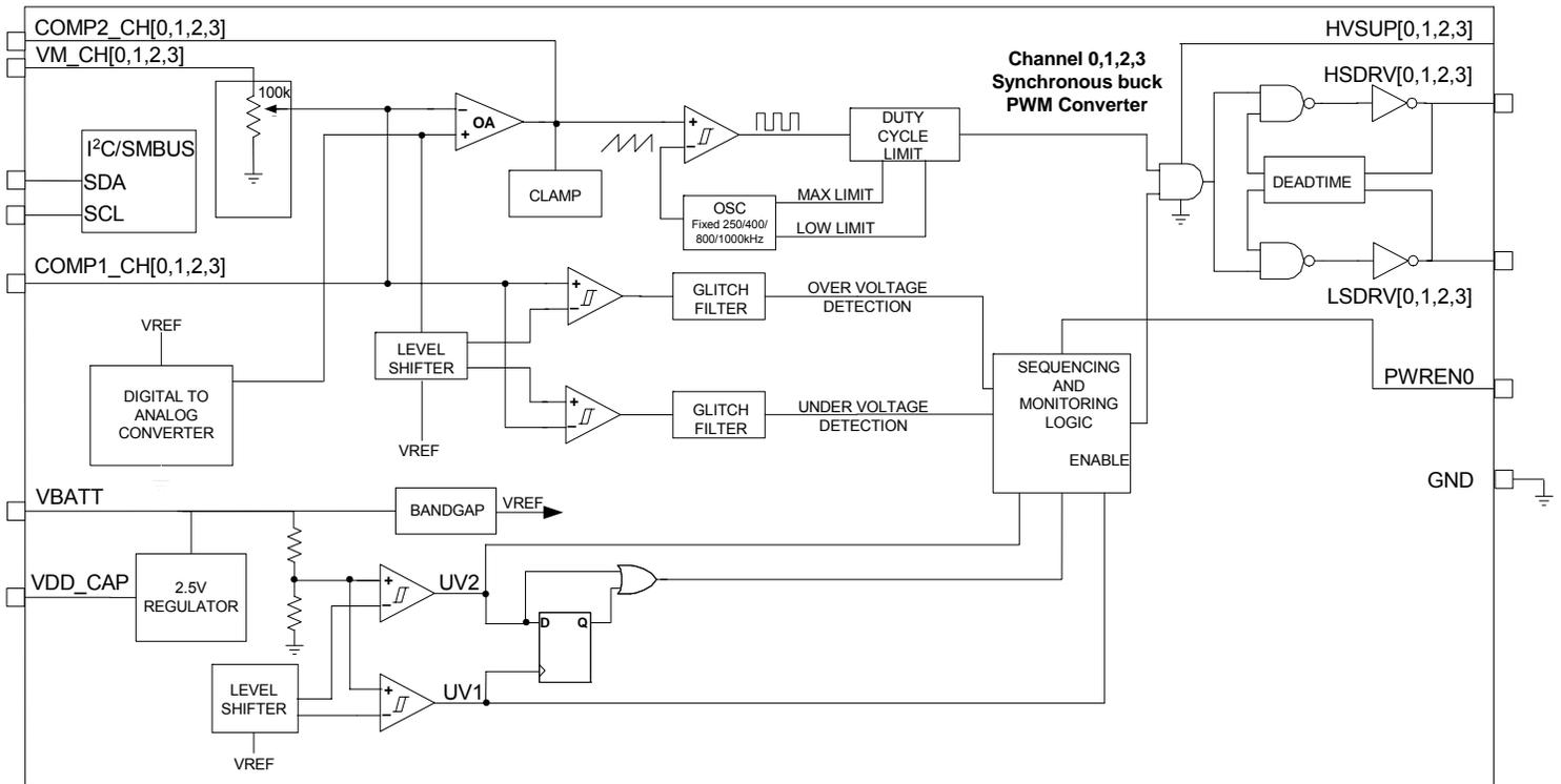
**Figure 3 –SMB113A/B and SMB117A internal block diagram. Programmable functional blocks include: level shifters, digital to analog converter and the VM\_CH[0,1,2,3] voltage dividers.**
