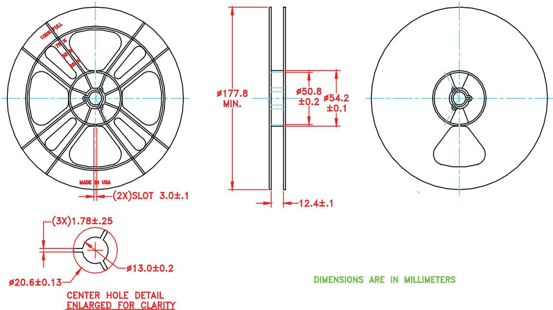
DIMENSIONS ARE IN MILLIMETERS
