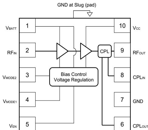
**Figure 1: Block Diagram**
