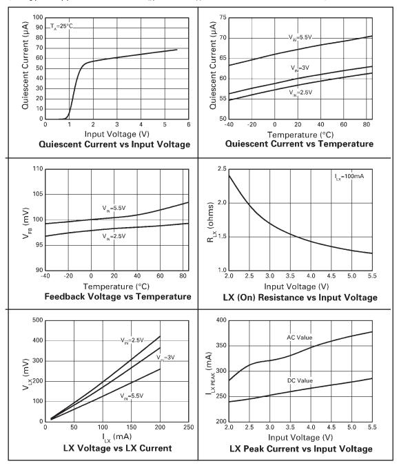
TYPICAL CHARACTERISTICS (For typical application circuit at  $V_{\rm IN}{=}3V$  and  $T_{\rm A}{=}25^\circ\text{C}$  unless otherwise stated)
