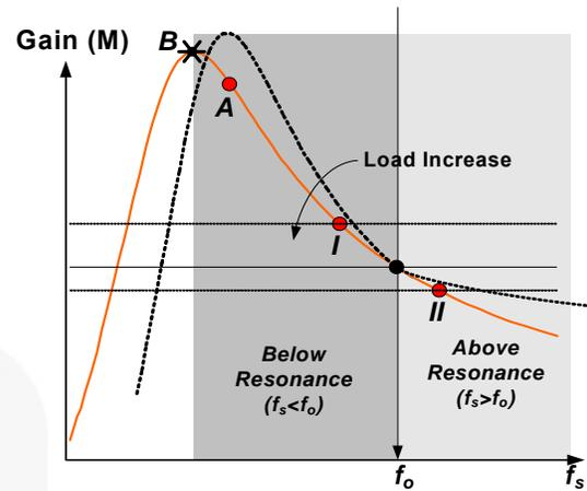
Figure 10. Operation Modes According to the Operation Frequency
