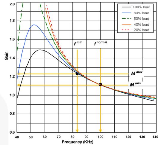
Figure 21. Gain Curve
