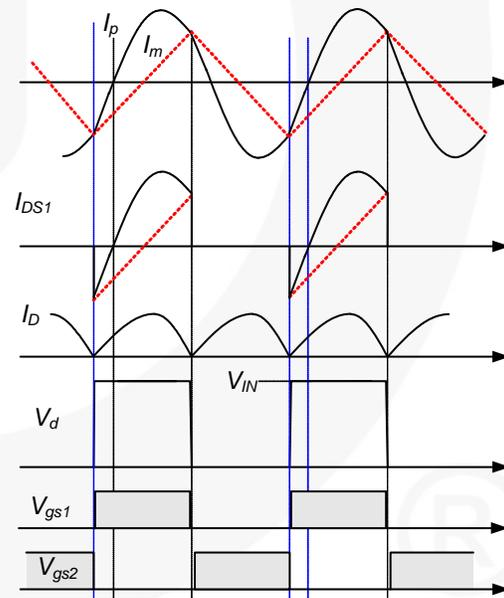
**Figure 4. Typical Waveforms of Half-Bridge LLC Resonant Converter**
