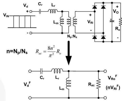
Figure 6. AC Equivalent Circuit for LLC Resonant Converter
