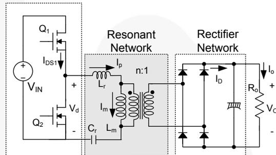
**Figure 3. Schematic of Half-Bridge LLC Resonant Converter**
