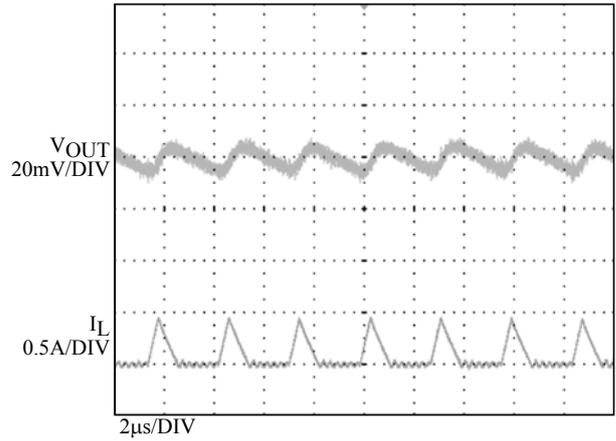
$I_{OUT} = 2\text{A}$  Operate waveform
