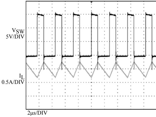
$I_{OUT} = 2\text{A}$  Output waveform
