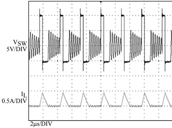
$I_{OUT} = 200\text{mA}$  Output waveform
