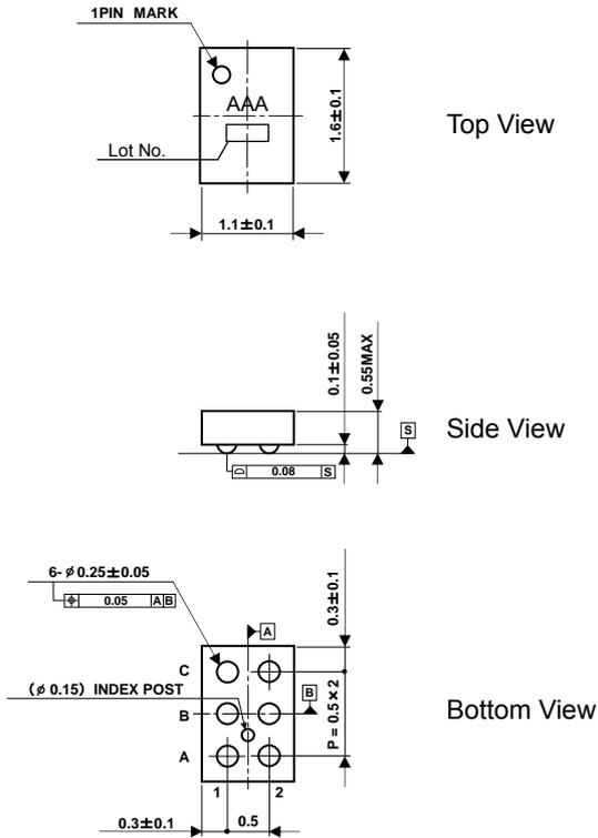
Fig.1 VCSP50L1 Package (Unit: mm)
