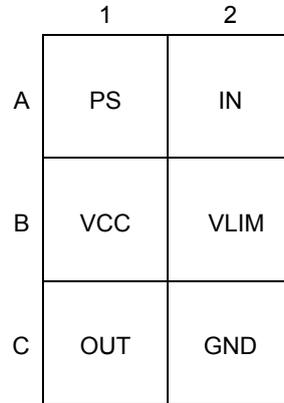
Fig.2 BD6883GUL Pin Arrangement (Top View)
