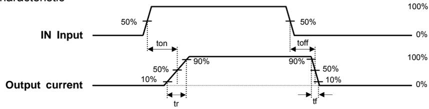
The voltage and current waveform show the turn on time, turn off time, rise time and fall time when input pulse was applied at IN.
