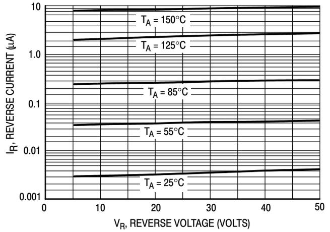
Figure 3. Leakage Current
