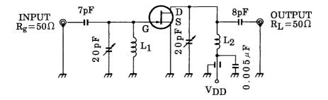
$L_1{:}~0.8~\text{mm}\phi~\text{A}_g$  plated Cu wire 3 turns, 10 mm ID, 10 mm length
