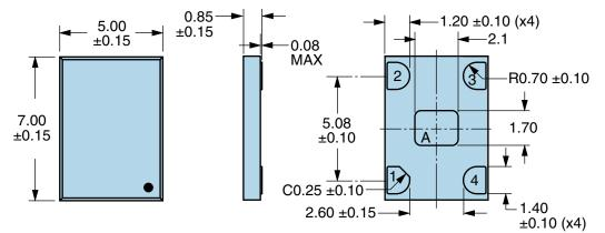
Note A: Center paddle is connected internally to oscillator ground (Pad 2).
