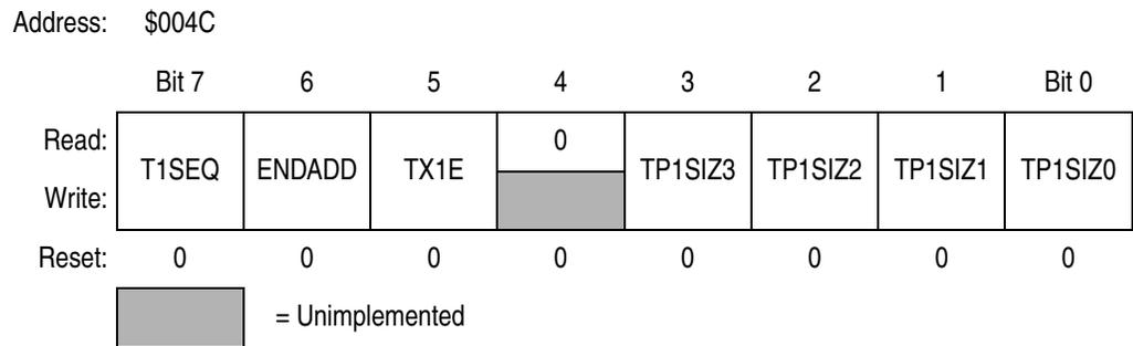
**Figure 9-16. USB Embedded Device Control Register 1 (DCR1)**
