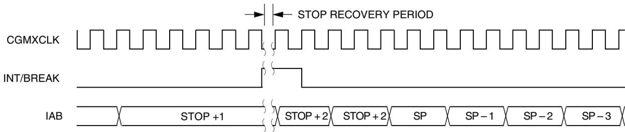
**Figure 7-19. Stop Mode Recovery from Interrupt or Break**
