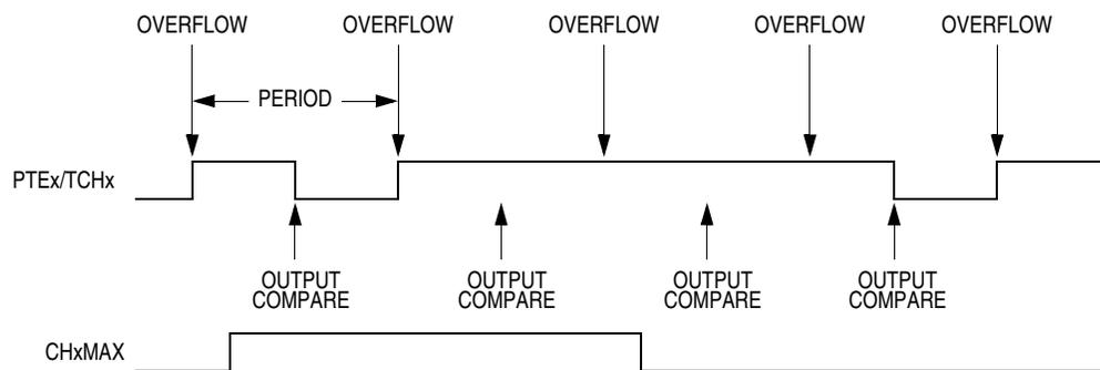
**Figure 11-8. CH<sub>x</sub>MAX Latency**
