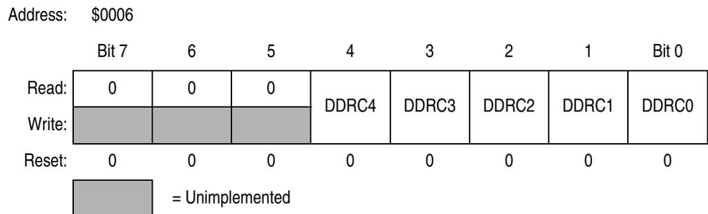
Figure 12-8. Data Direction Register C (DDRC)
