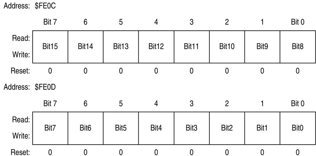
Figure 16-3. Break Address Registers (BRKH and BRKL)
