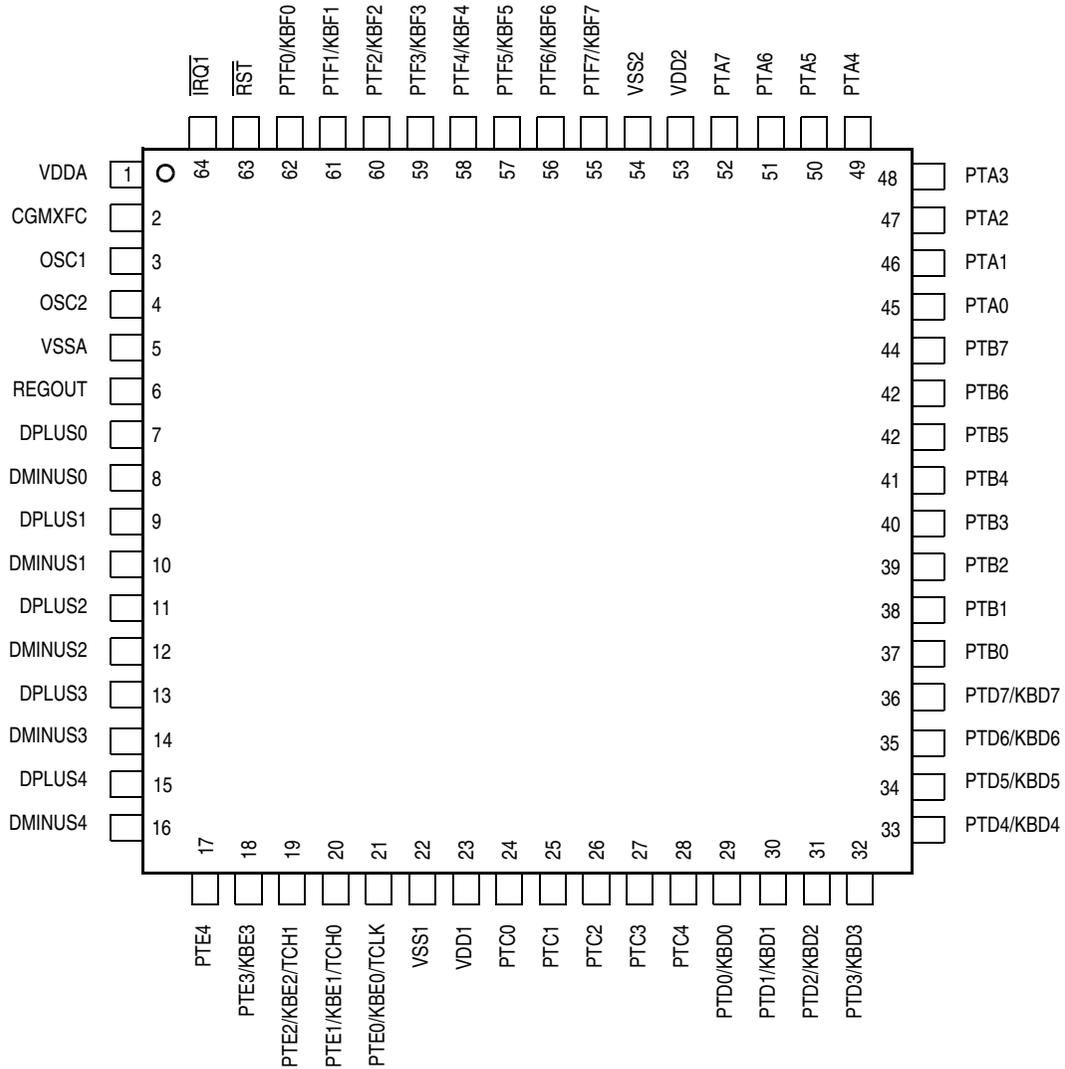
Figure 1-2. 64-Pin QFP Pin Assignment (Top View)
