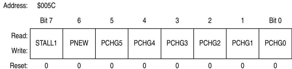
**Figure 9-9. USB HUB Control Register 1 (HCR1)**
