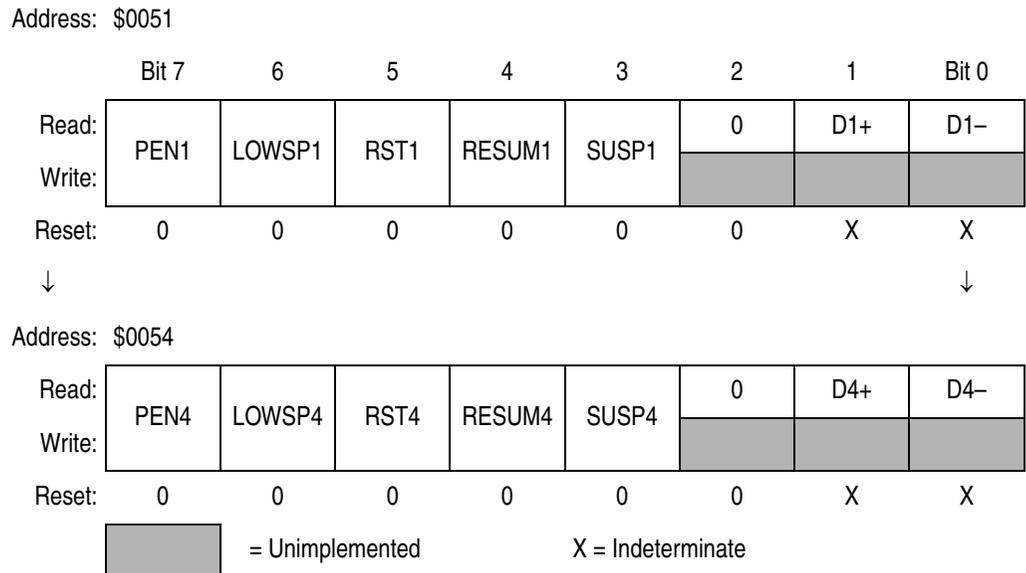
**Figure 9-3. USB HUB Downstream Port Control Registers (HDP1CR-HDP4CR)**
