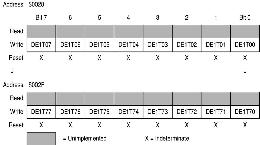
**Figure 9-20. USB Embedded Device Endpoint 0 Data Register (UE0D0-UE0D7)**
