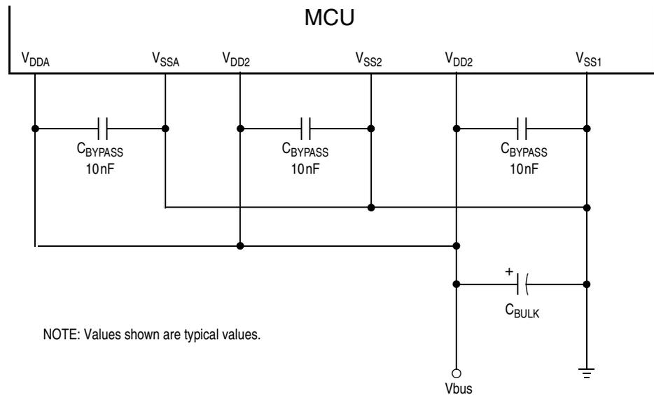
Figure 1-4. Power Supply Bypassing
