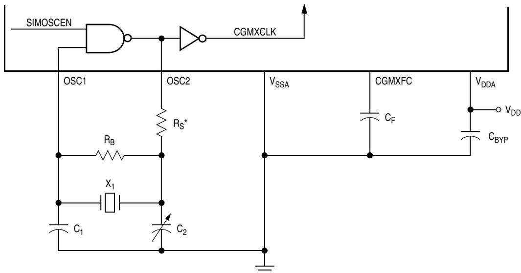
\* $R_S$  can be zero (shorted) when used with higher-frequency crystals. Refer to manufacturer's data.
