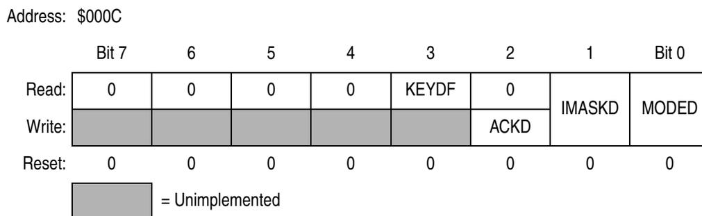
**Figure 15-2. Port-D Keyboard Status and Control Register (KBDSCR)**
