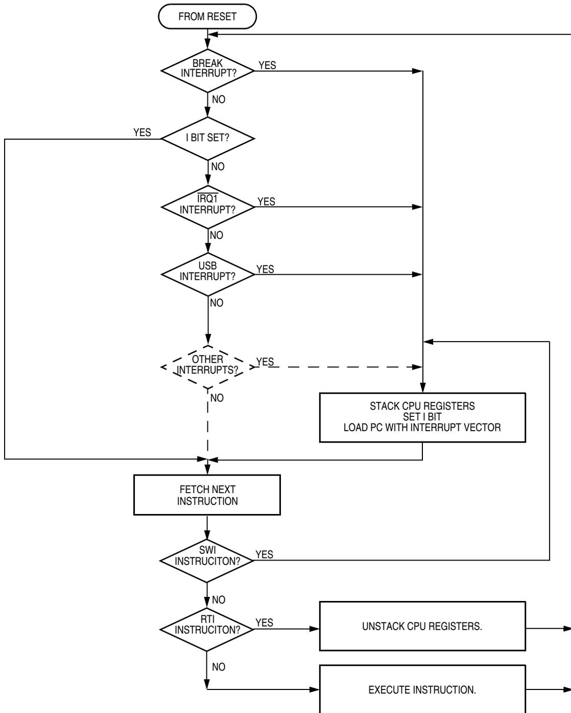
Figure 7-8. Interrupt Processing
