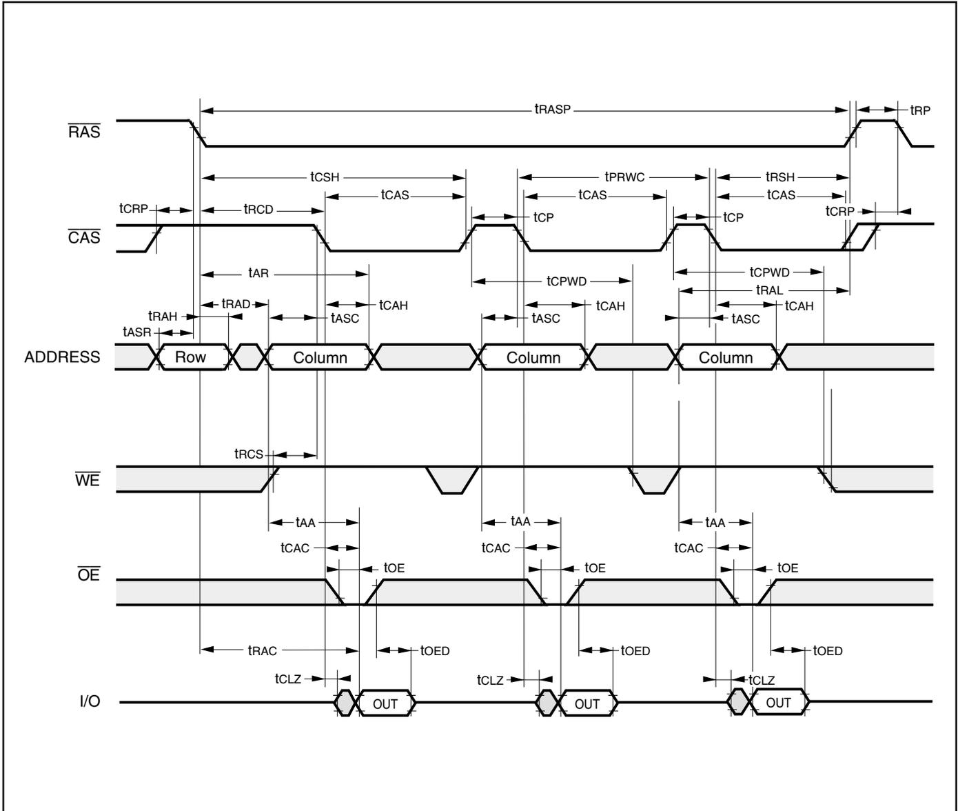
**FAST-PAGE-MODE READ WRITE CYCLE (LATE WRITE and READ-MODIFY-WRITE Cycles)**
