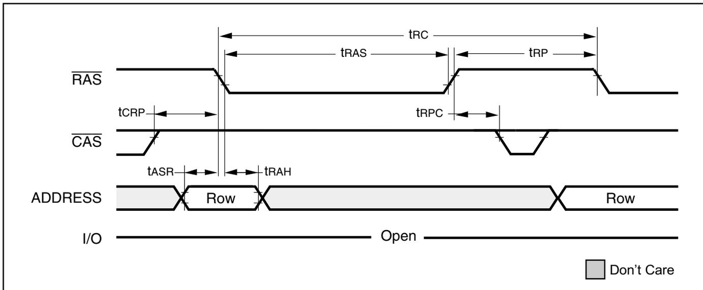
**$\overline{\text{CBR}}$  REFRESH CYCLE** (Addresses;  $\overline{\text{WE}}$ ,  $\overline{\text{OE}}$  = DON'T CARE)
