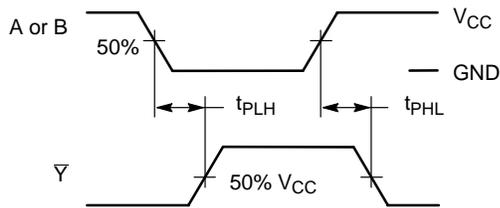
Figure 3. Switching Waveform
