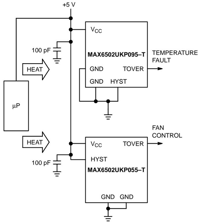
Figure 2. Fan Control Circuit with Over Temperature Alert
