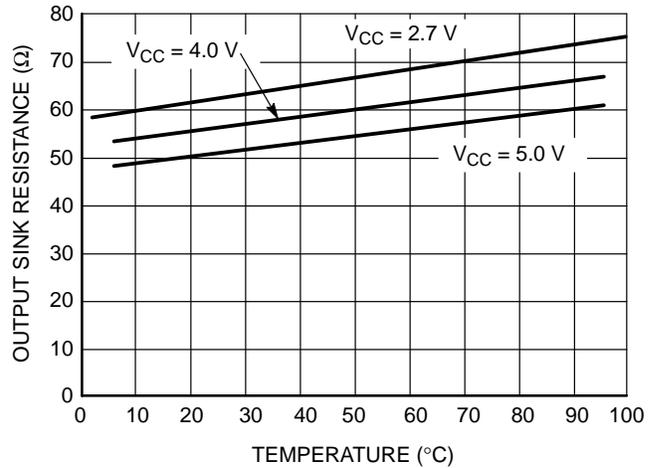
Figure 7. Output Sink Resistance vs. Temperature
