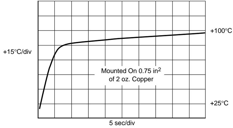
**Figure 9. SOT-23 Thermal Step Response in Perfluorinated Fluid**
