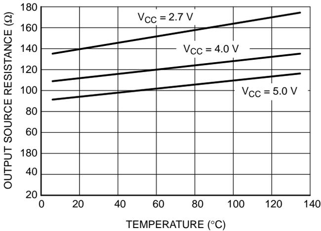
Figure 6. MAX6502 Output Source Resistance vs. Temperature
