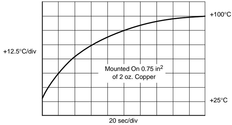
**Figure 10. SOT-23 Thermal Step Response in Still Air**
