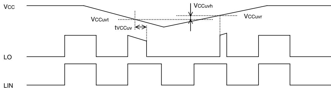
If Vcc supply voltage drops below UV trip voltage ( $VCCuvt = VCCuvt - VCCuvh$ ) for Vcc supply UV filter time, output signal becomes "L". As soon as Vcc supply voltage rises over UV reset voltage, output signal HO becomes "H" if input signal is "H".
