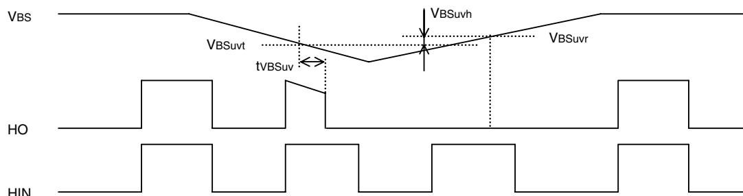
**HIGH VOLTAGE HALF BRIDGE DRIVER****3. Allowable Supply Voltage Transient**
