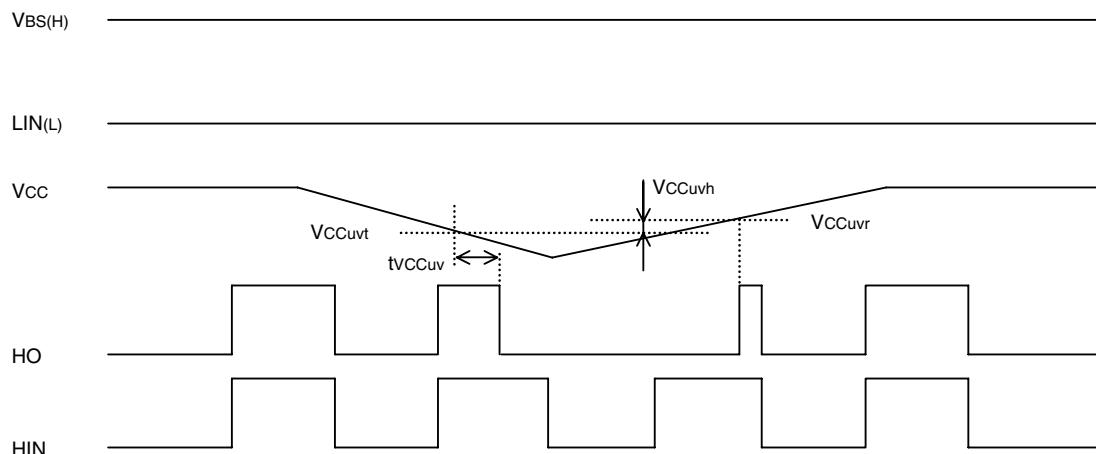
If VBS supply voltage drops below UV trip voltage ( $VBSuvt = VBSuvt - VBSuvh$ ) for VBS supply UV filter time, output signal becomes "L". As soon as VBS supply voltage rises over UV reset voltage, output signal HO becomes "H" at following "H" edge of input signal.
