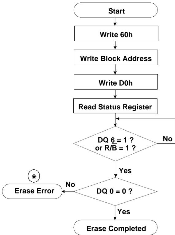
\* : If erase operation results in an error, map out the failing block and replace it with another block.
