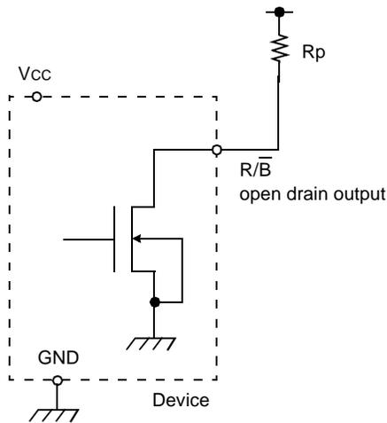
$$R_p = \frac{V_{cc}(\text{Max.}) - V_{OL}(\text{Max.})}{I_{OL} + \sum I_L} = \frac{2.9V}{8\text{mA} + \sum I_L}$$
