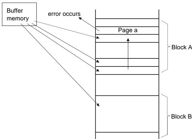
When the error happens with page "a" of Block "A", try to write the data into another Block "B" from an external buffer. Then, prevent further system access to Block "A" (by creating a "invalid block" table or other appropriate scheme.)
