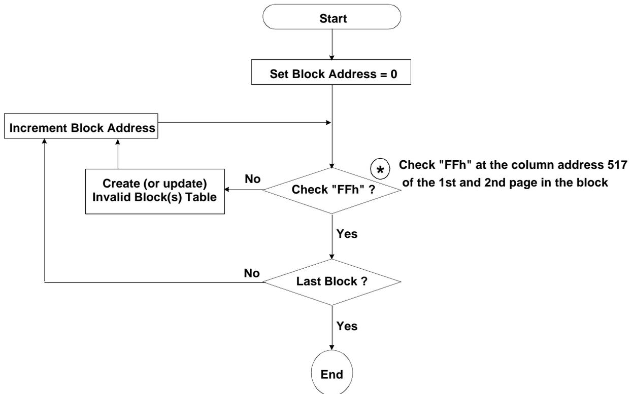
Figure 10. Flow chart to create invalid block table
