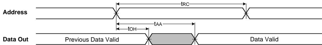
**TIMING WAVEFORM OF READ CYCLE(2)**( $\overline{ZZ}=\overline{WE}=V_{IH}$ )
