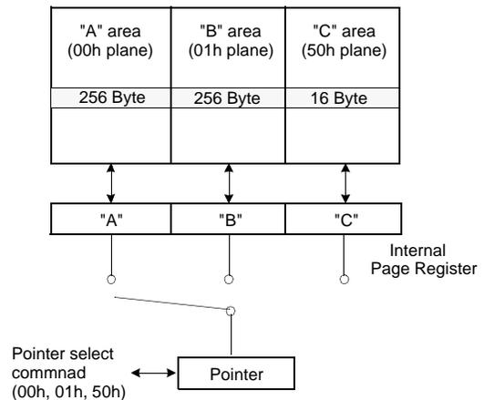
**Figure 15. Block Diagram of Pointer Operation**
