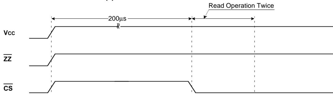
**TIMING WAVEFORM OF POWER UP(2)(No Dummy Cycle)**
