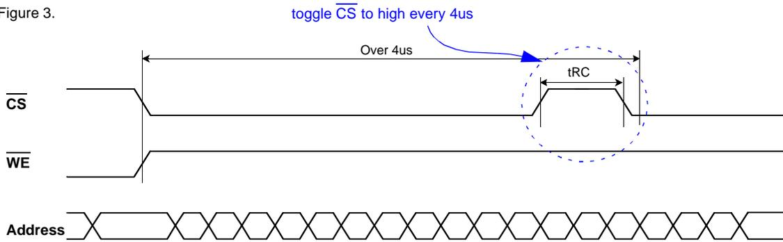
Write operation have similar restricted operation with Read. If your system have a timing which sustain invalid states over 4us at write mode and system have continuous write signal with Min. tWC over 4us like Figure 4.
