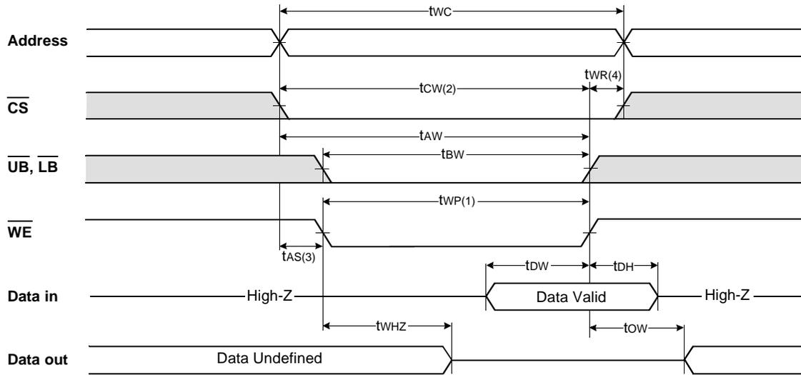
**TIMING WAVEFORM OF WRITE CYCLE(2)**( $\overline{CS}$  Controlled,  $\overline{ZZ}=V_{IH}$ )
