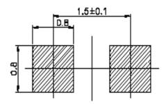
**Notes:**Tolerances Unless Dimension ±0.1mm,Angle±0.5",Unit=mm
