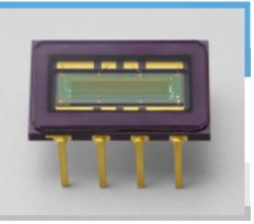
S9227 is a small CMOS linear image sensor designed for image input applications. Signal charge is integrated on all pixels simultaneously and then read out at high speeds of 5 MHz.
