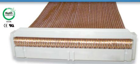
Cicoil's ribbon cables are constructed using Ultra High Flex 28 AWG, finely stranded wire, and our exclusive silicone extrusion process for a strong, flexible, clear cable. Our ribbon cables meet the standard ribbon cable dimensions, and they can be used with any standard Insulation Displacement Connectors (IDC). The wire spacing ('pitch') is set at .050" for the English version, or 1mm for the metric version.
