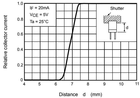
**Relative Positioning Of Shutter And Device**
