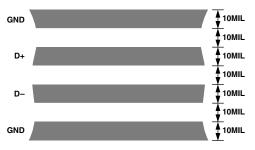
Figure 6. Arrangement of Signal Tracks
