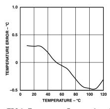
TPC 2. Temperature Error vs. Actual Temperature Using 2N3906
