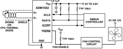
Figure 7. Typical Application Circuit
