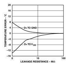
TPC 1. Temperature Error vs. Leakage Resistance
