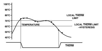
Figure 5. Operation of the THERM Output
