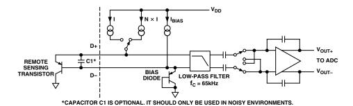
Figure 2. Input Signal Conditioning
