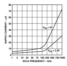
TPC 8. Standby Supply Current vs. Clock Frequency
