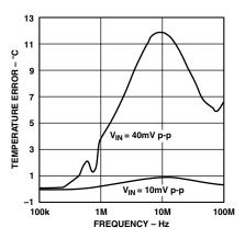
TPC 3. Temperature Error vs. Differential Mode Noise Frequency
