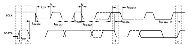
Figure 1. Diagram for Serial Bus Timing
