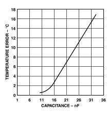
TPC 5. Temperature Error vs. Capacitance between D+ and D-
