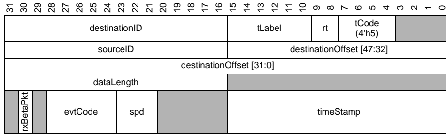
Figure 3-5 RxRdReqDB - Block Read Request Receive Packet Format
