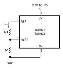
Figure 2. Programming the HYST Pin
