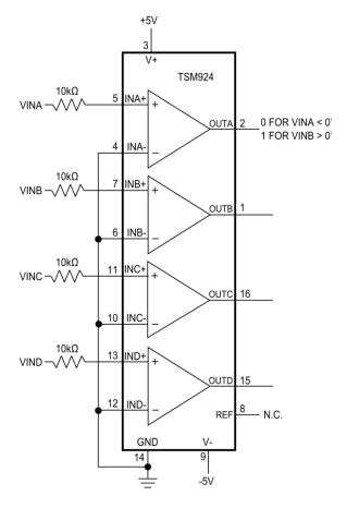
Figure 7. Level Shifter: ±5V Input into CMOS output
