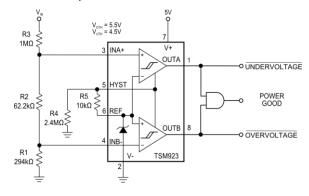
Figure 5. Window Detector
