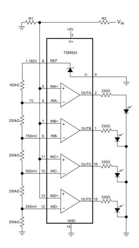
Figure 6. Bar-Graph Level Gauge
