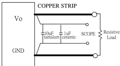
Note: Use a 10 $\mu$ F tantalum and 1 $\mu$ F capacitor. Scope measurement should be made using a BNC connector.
