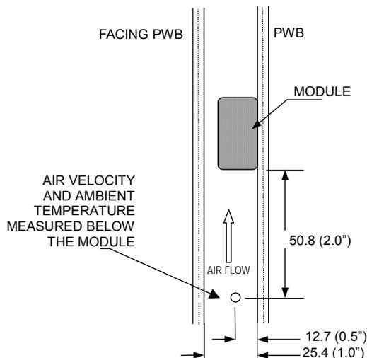
Figure 32: Wind tunnel test setup figure
