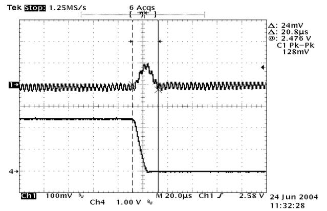
Figure 22: Typical transient response to step load change at 0.5A/μS from 50% to 0% of Io, max at 5.0Vin, 2.5V out (measurement with a 1uF ceramic and a 10μF tantalum)
