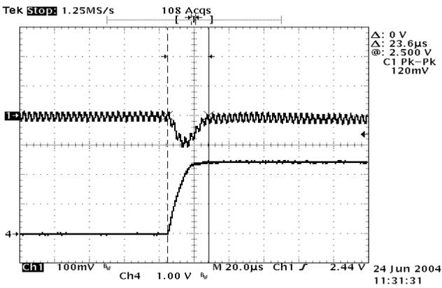
Figure 21: Typical transient response to step load change at 0.5A/μS from 0% to 50% of Io, max at 5.0Vin, 2.5V out (measurement with a 1uF ceramic and a 10μF tantalum)
