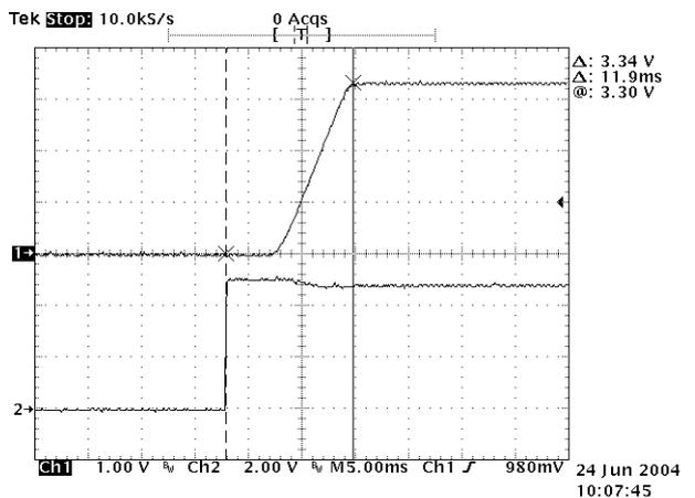
Figure 18: Remote turn on delay time at 5.0vin, 3.3V/10A out
