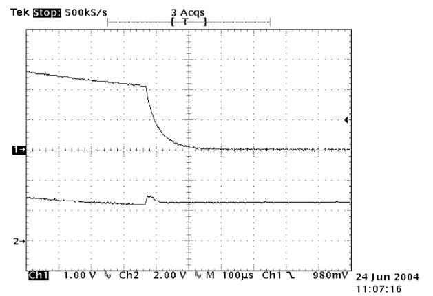
Figure 16: Power off waveform 5.0vin, 3.3V/10A out with application of Vin
