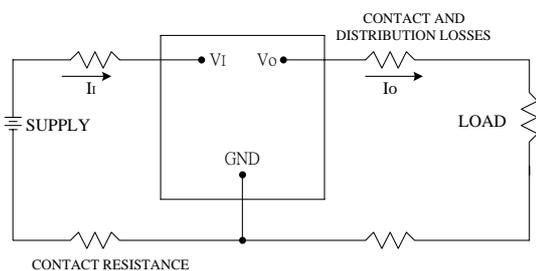
**Figure 25:** Output voltage and efficiency measurement test setup
