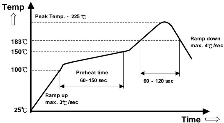
Note: All temperature refers to assembly application board, measured on the land of assembly application board.
