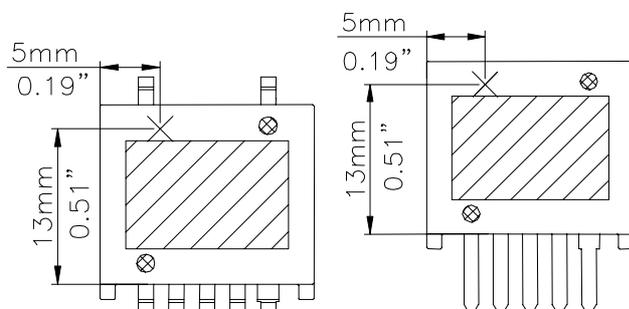
Figure 33: Temperature measurement location
