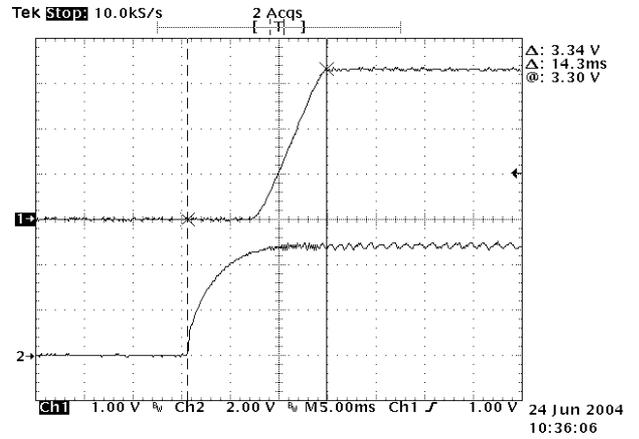
Figure 20: Turn on delay at 5.0Vin, 3.3V/10A out with application of Vin
