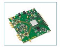
DAC1408D750 demonstration board, for easy connection to Altera, Xilinx or Lattice evaluation kit
