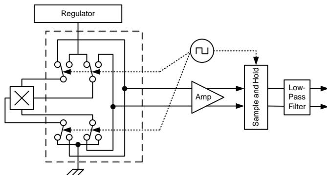
Figure 2. Chopper stabilization circuit (dynamic quadrature offset cancellation)
