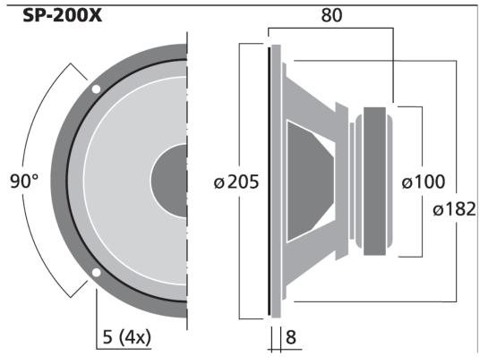
Hi-fi Full Range Speaker, with Dual Cone, with one-piece rubber gasket, very good linearity and high efficiency, an excellent full range speaker of high power capability which can be used as midrange speaker in PA systems of special sound requirements or in large column speakers.
