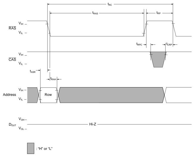
NOTE:  $\overline{\text{WE}}$ ,  $\overline{\text{OE}}$  and  $D_{\text{IN}}$  are "H" or "L"
