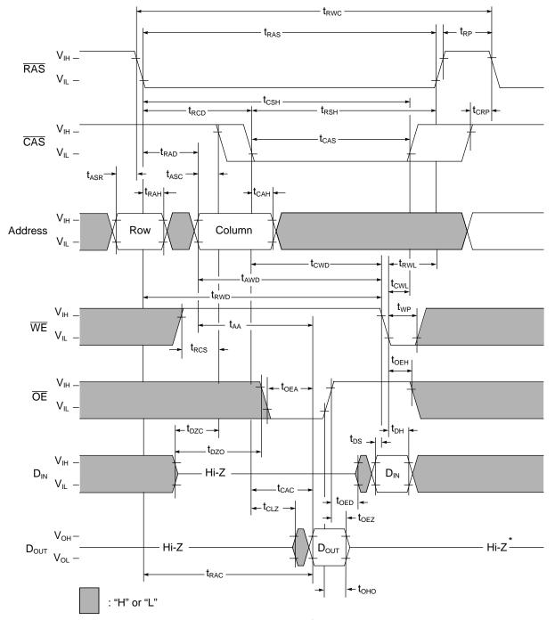
$t_{OEH}$  greater than or equal to  $t_{CWL}$
