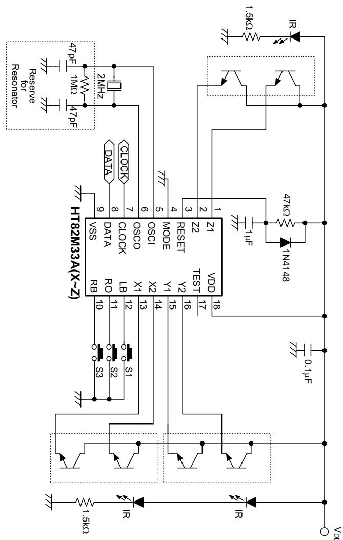
HT82M33A 3D PS2 mouse (This application circuit is for reference only)
