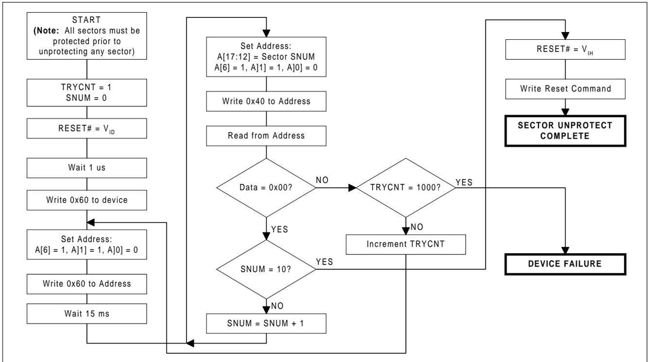
Figure 2. Sector Unprotect Algorithm
