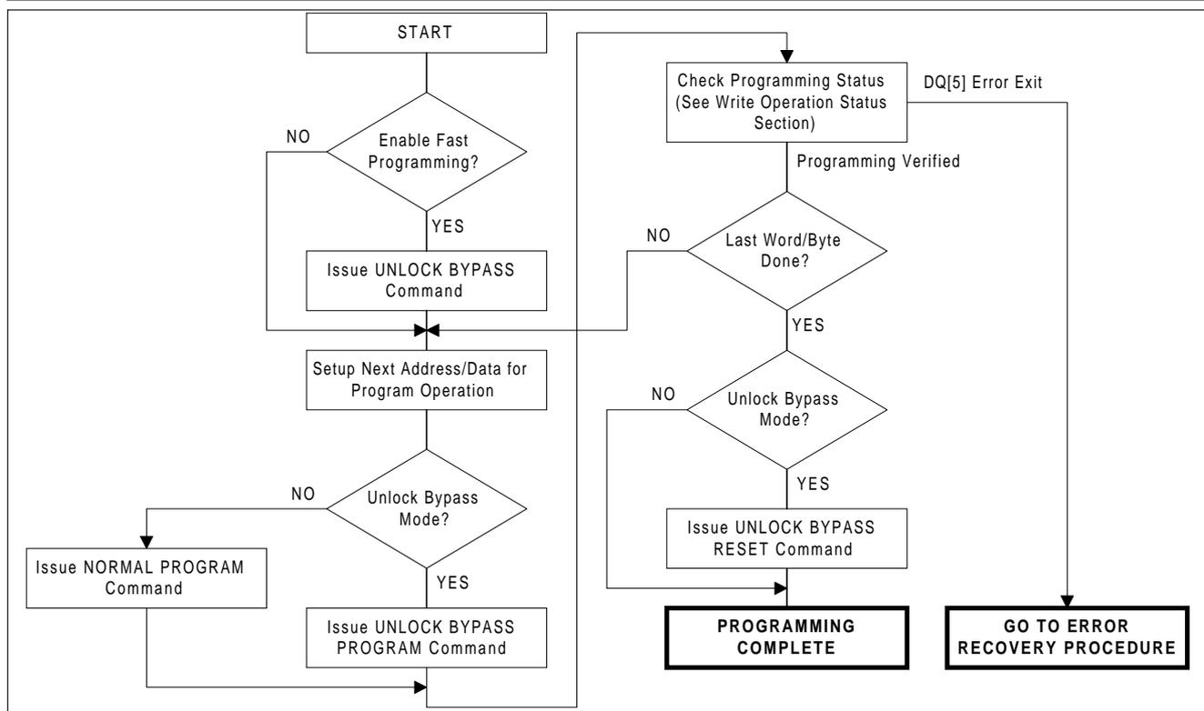
**Figure 4. Normal and Unlock Bypass Programming Procedures**
