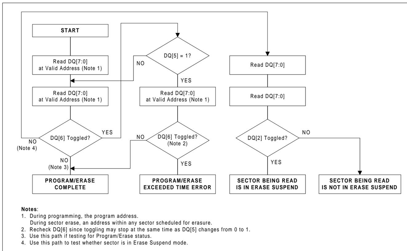
Figure 8. Toggle Bit I and II Test Algorithm
