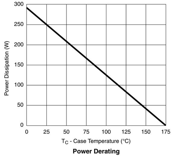
\*The power dissipation  $P_D$  is based on  $T_{J(max)} = 175\text{ °C}$ , using junction-to-case thermal resistance, and is more useful in settling the upper dissipation limit for cases where additional heatsinking is used. It is used to determine the current rating, when this rating falls below the package limit.
