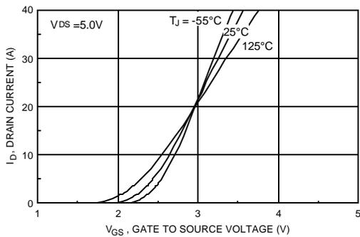
Figure 5. Transfer Characteristics.
