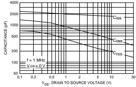
Figure 8. Capacitance Characteristics.
