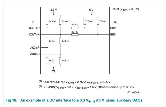
The constraints to adjust the interface are the output compliance range of the DAC and the auxiliary DACs, the input common-mode level of the AQM, and the range of offset correction.
