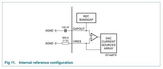
This configuration is optimum for temperature drift compensation because the bandgap reference voltage can be matched to the voltage across the feedback resistor.
