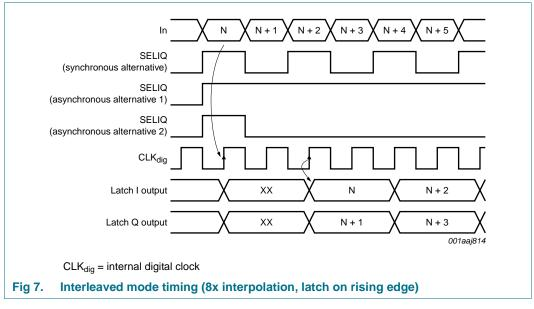
The SELIQ signal can be either synchronous or asynchronous (single rising edge, single pulse). The first data following the SELIQ rising edge is sent in channel I and following data is sent in channel Q. After this, data is distributed alternately between these channels.
