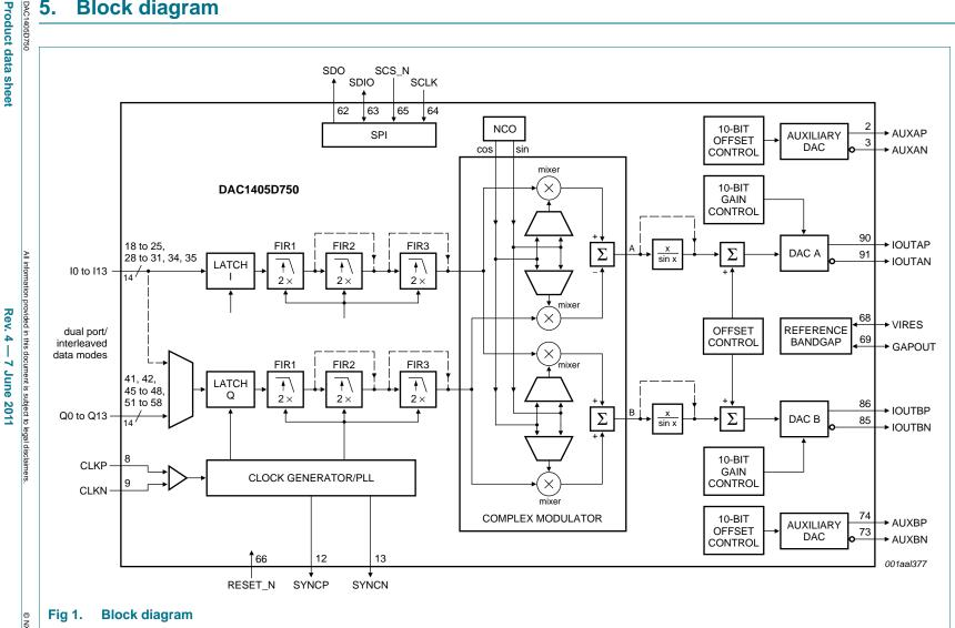
Dual 14-bit DAC, up to 750 Msps; 4× and 8× interpolating DAC1405D750
