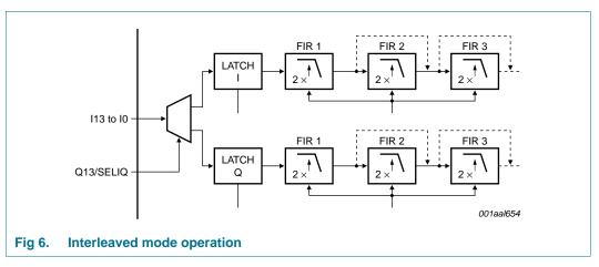
In Interleaved mode, both DACs use the same data input at twice the Dual-port mode frequency. Data enters the latch on the rising edge of the internal clock signal. The data is sent to either latch I or latch Q, depending on the SELIQ signal.
