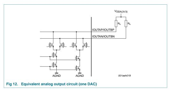
The cascode source configuration increases the output impedance of the source, thus improving the dynamic performance of the DAC by introducing less distortion.
