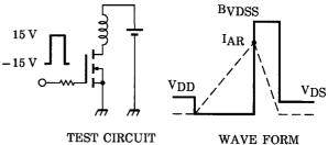
$$\begin{array}{l} R_G = 25 \ \Omega \\ V_{DD} = 25 \ V \!\!\!, \ L = 428 \ \mu H \end{array} \qquad \qquad \\ EAS = \frac{1}{2} \cdot L \cdot I^2 \cdot \left( \frac{BVDSS}{BVDSS - VDD} \right) \end{array}$$
