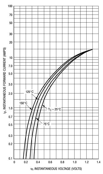
Figure 1. Typical Forward Voltage, Per Leg
