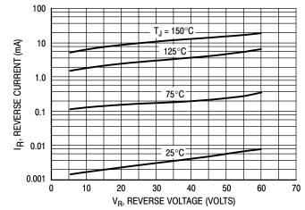
\*The curves shown are typical for the highest voltage device in the voltage grouping. Typical reverse current for lower voltage selections can be estimated from these curves if  $V_R$  is sufficient below rated  $V_R$ .
