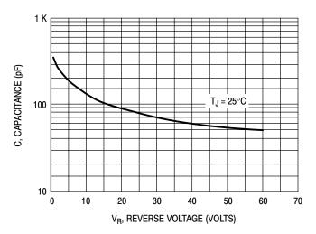
Figure 6. Typical Capacitance, Per Leg
