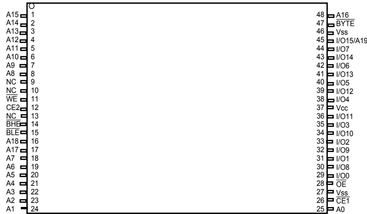
Figure 3. 48-pin TSOP I (512 K × 16/1 M × 8) (Top View) [1, 3]
