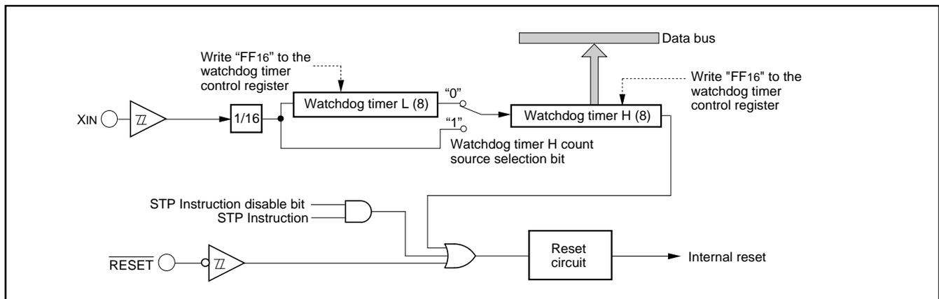
Fig. 41 Block diagram of watchdog timer
