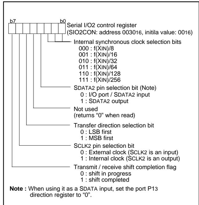
Fig. 35 Structure of serial I/O2 control registers
