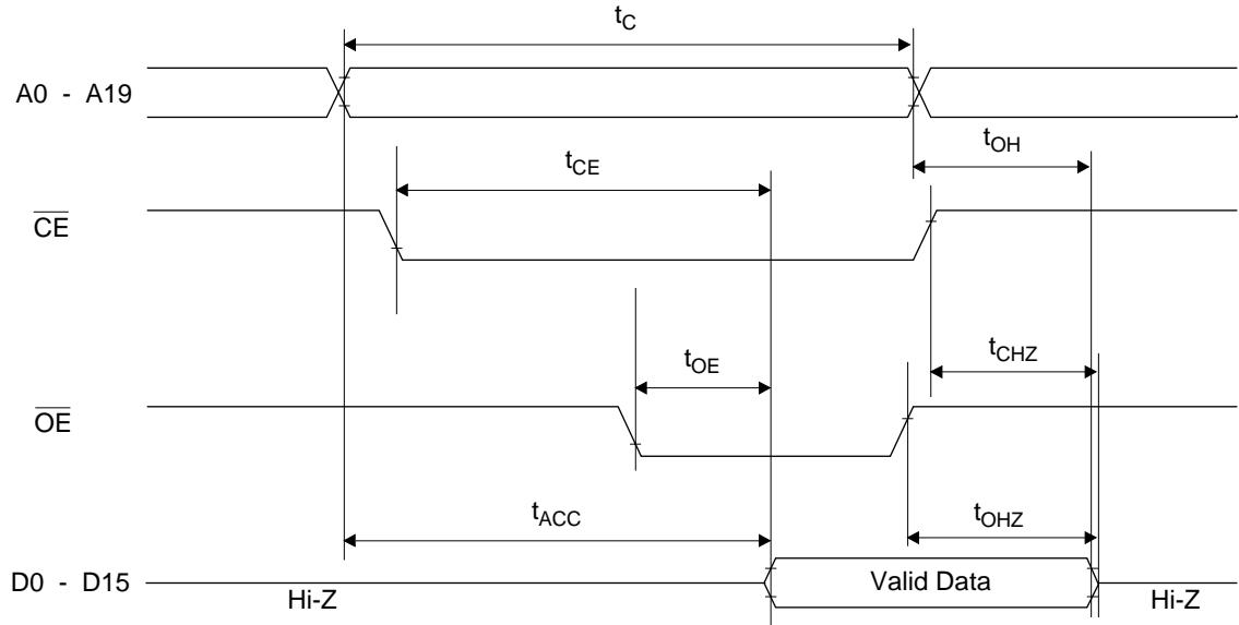
**8-Bit Read Mode ( $\overline{\text{BYTE}}=V_{IL}$ )**
