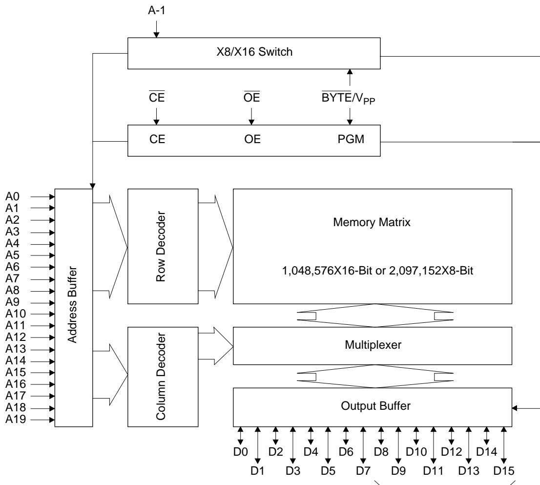
In 8-bit output mode, these pins are three-stated and pin D15 functions as the A-1 address pin.
