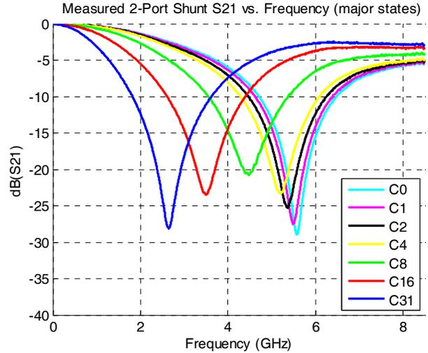
**Figure 12. Measured Self Resonance Frequency vs State**
