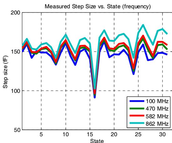
Figure 7. Measured Series S<sub>11</sub>/S<sub>22</sub> (major states)
