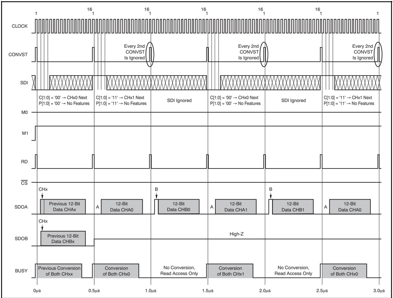
Figure 17. Mode II Timing Diagram (M0 = 0; M1 = 1)
