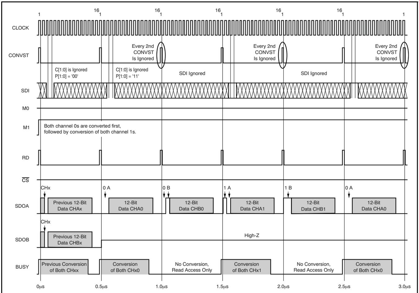
Figure 19. Mode IV Timing Diagram (M0 = 1 ; M1 = 1)
