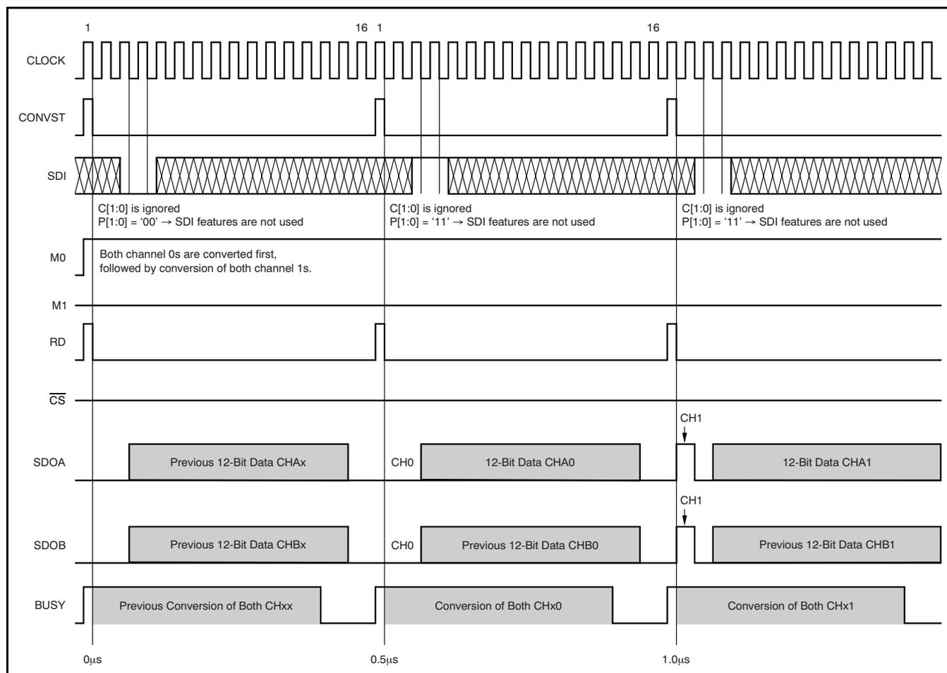
Figure 18. Mode III Timing Diagram (M0 = 1; M1 = 0)
