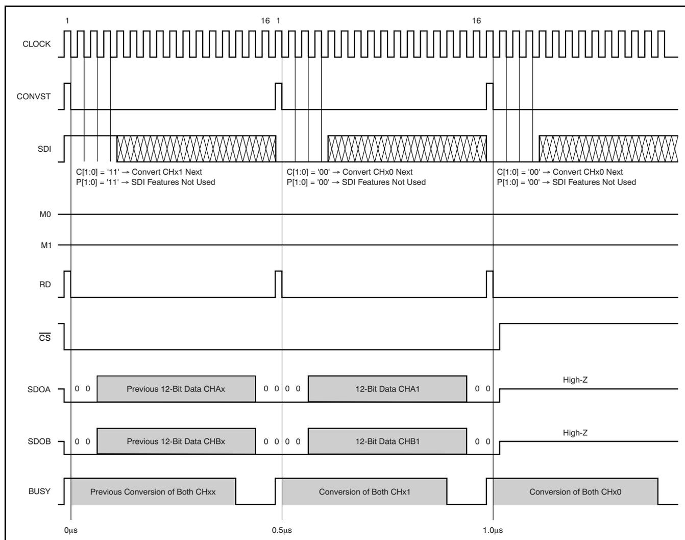
Figure 16. Mode I Timing Diagram (M0 = 0; M1 = 0)
