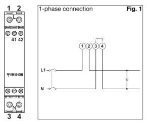
**NOTE:** The 3 and 4 terminals, in the instrument, are wired together
