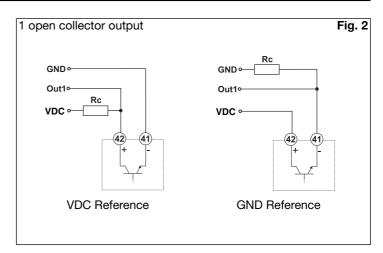
The load resistances (RC) must be designed so that the close contact current is lower than 100mA; the VDC voltage must be lower than or equal to 30VDC.
