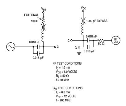
Figure 1. NF, G<sub>pe</sub> Measurement Circuit 20–200
