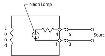
Since this is a double break device, one side of the electrical source should be connected to terminal 3 and the other side to terminal 6. The electrical load should be connected between terminals 1 and 4.
