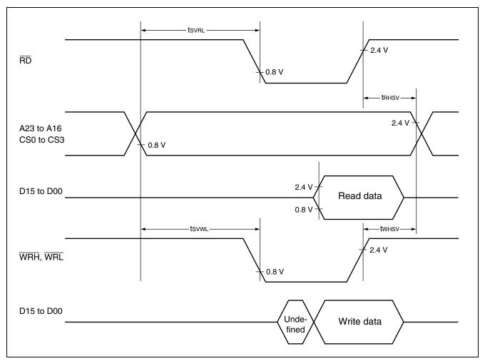
Note : Due to the configuration of the internal bus, the chip select output signals are changed simultaneously and therefore may cause the bus conflict conditions. AC cannot be warranted between the ALE output signal and the chip select output signal.
