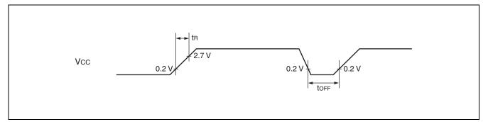
Note : Rapid fluctuations in power supply voltage may trigger a power-on reset in some cases. As shown below, when changing supply voltage during operation, it is recommended that voltage changes be suppressed and a smooth restart be applied.
