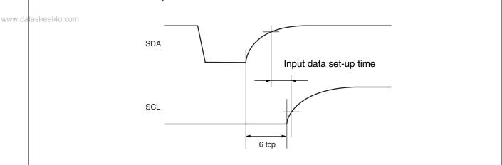
Note : The rating of the input data set-up time in the device connected to the bus cannot be satisfied depending on the load capacitance or pull-up resistor. Be sure to adjust the pull-up resistor of SDA and SCL if the rating of the input data set-up time cannot be satisfied.
