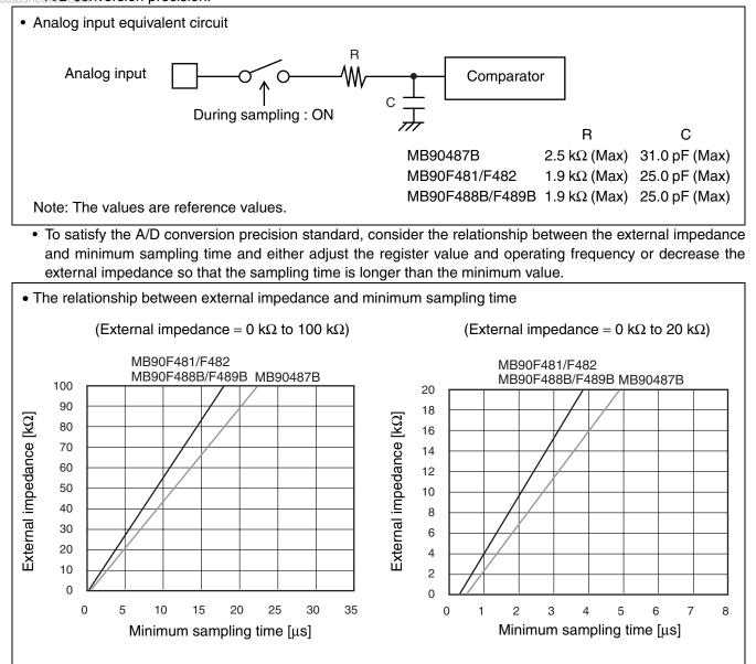
• If the sampling time cannot be sufficient, connect a capacitor of about 0.1  $\mu$ F to the analog input pin.
