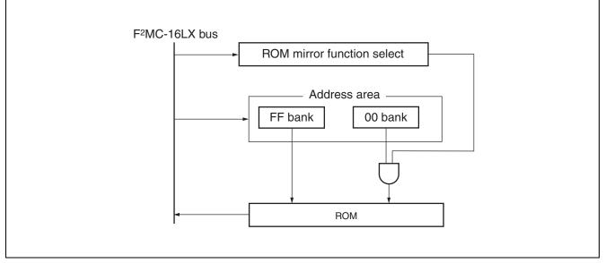
Note : Do not access ROM mirror function selection register (ROMM) on using the area of address 004000<sup> H</sup> to 00FFFF<sub>H</sub> (008000<sup> H</sup> to 00FFFF<sub>H</sub>) .
