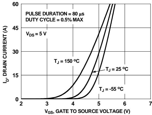
**Figure 5. Transfer Characteristics**
