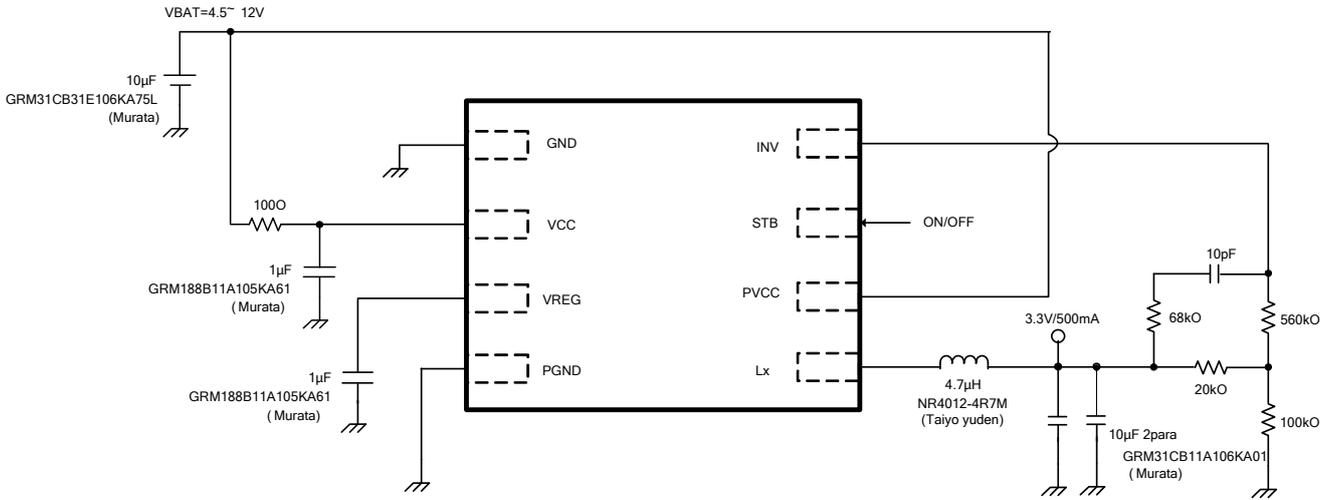
Fig.32 Reference application diagram2
