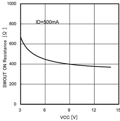
Fig.13. Pch FET ON resistance power supply property
