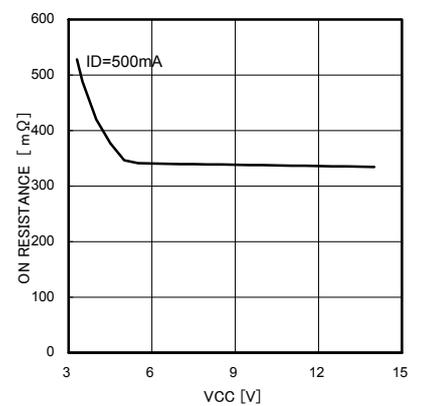
Fig.11. Nch FET ON resistance power supply property
