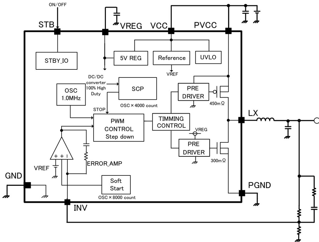
Fig.2 Block diagram
