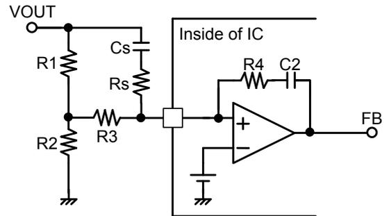
Fig.51 Example of phase compensation setting
